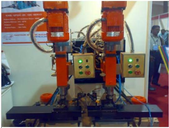
**Auto-Feed Drilling and Auto-Feed Tapping machine.**
